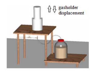
Figure 1. Bench digesters used in this experiment and a scheme of the set detailing the gasholder displacement [From: Inoue (2008)].
