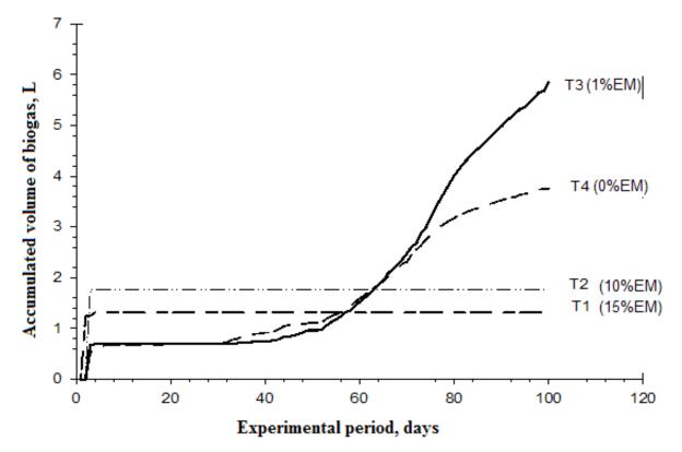
**Figure 2.** Estimates for accumulated biogas production along the experimental period, for each treatment [(T1 (15% EM), T2 (10% EM), T3 (1% EM) and T4 (0% EM)].
