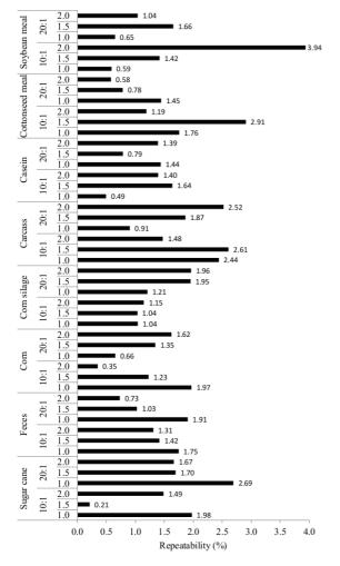
**Figure 1**. Standardized repeatability for the different low- and high-nitrogen materials according to the salt-to-metal catalyst ratios and amounts of digestion mixture.
