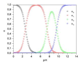
Figure 4. Species distribution diagram of amoxicillin. Graphic generated from electronic worksheet TitGer.
