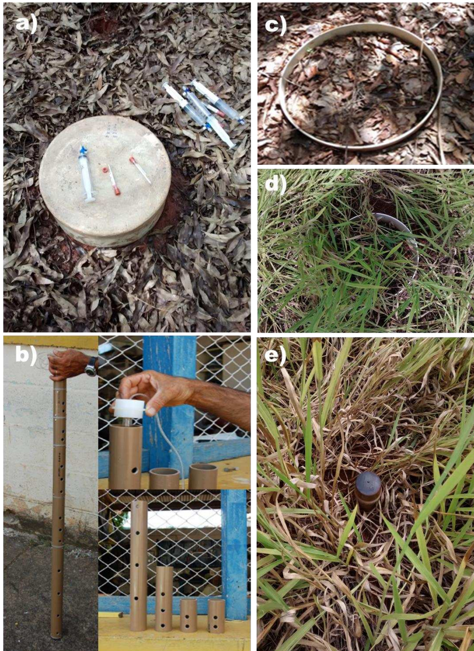
Supplementary material 2. Static PVC chambers (0.30-m height x 0.4-m diameter) used to measure soil surface CO 2 -C and CH 4 -C fluxes in the Cerrado (c), pasture (d) and eucalypt (a) and PVC (1.0-m height x 0.025-m diameter) access tube with subdivisions used to collect soil air in the layers 0.0-0.1, 0.1-0.2, 0.2-0.4, 0.4-0.6, 0.6-1.0 m (b and e).
