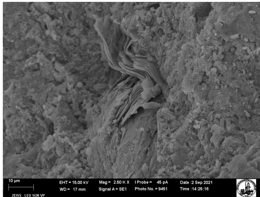
Fig. 19. Portlandite decomposition in C50 after exposure to 600 °C.
