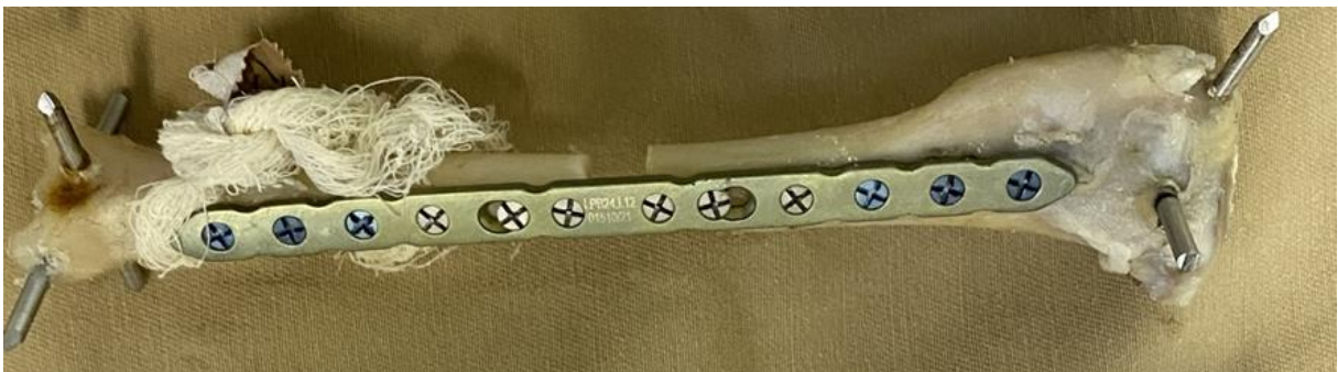
Figure 3 – Correct insertion of the screws in LCP with all locking screws heads above the surface of the plate.
