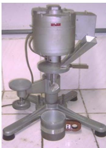
Figura 11 – Stein Breakage Tester, modelo CK2.
